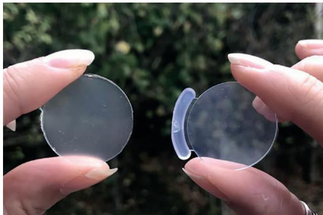
*The image shows two PP samples one containing a clarifying agent (right) and the other in its natural state (left). The sharpness of the image viewed through the sample on the right appears much clearer than that of the one on the left.*
